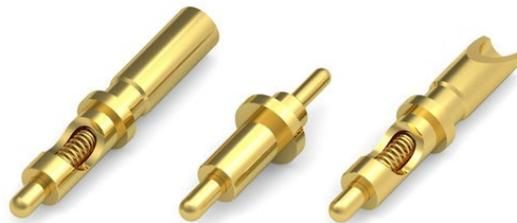
Pogo Pins are always a consideration for data transmission and can be a reliable connection for power and low speed data signals. However, this 40-year old technology is not designed to reliably transmit speeds above USB2 speeds of 480Mbps. Additionally, the pogo pin design requires tight alignment between the pin and the pad, where the connection is made. This is especially true when trying to transmit 1Gbps+ data rates over a pogo pin connection.
